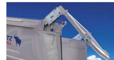
The functioning of the hydraulic rear wall can be controlled for voluminous bulk material or controlled partial unloading by means of the S.KI control app.
