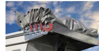
**Time gain when loading:** An app is used to open or close the electric sliding tarpaulin in only 25 seconds. Tipping can also be performed with the trough covering only partially opened.
