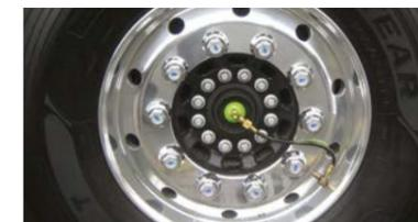
The tyre pressure monitoring and re-pressurisation system also enables continued and limited travel to the workshop in the case of slow pressure loss.
